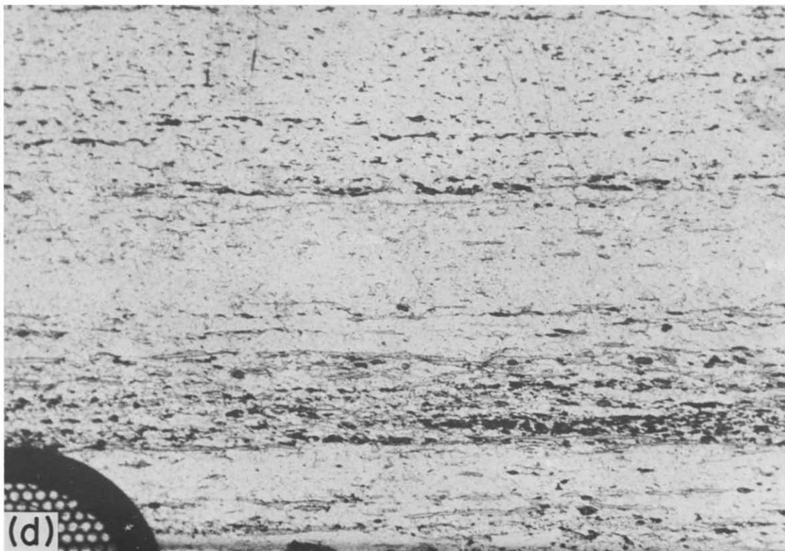
Fig. 7. (c) XN view of MR12(ii) illustrating the quartz microstructures including: complete recrystallization, smaller grain size in association with the micas and accessories, irregular grain boundaries, but with evidence of strain-driven grain boundary migration ('relaxation') as micas are enclosed by some grains. (d) PPL view of MR12(ii), illustrating the debris like trails of spindly white micas, epidotes and iron ore, within the strongly mylonitic flaggy rock.
